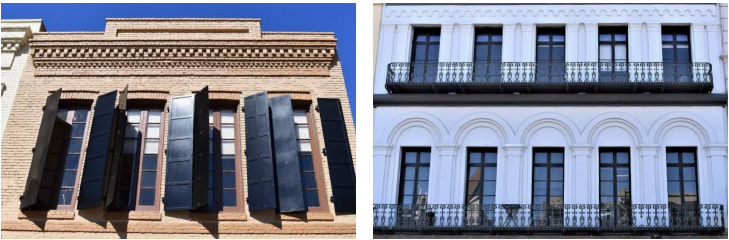
Figure 21: Windows and doors should be scaled and arranged to relate to the pattern of tall, vertically oriented, evenly spaced windows and doors at historic buildings.
